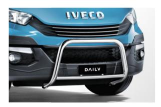
To increase safety, as an additional frontal protection for the bumper, it is possible to install the pushbar from the IVECO Accessories Line, with European certification, which can **increase the active and passive protection** of the vehicle and pedestrians.
